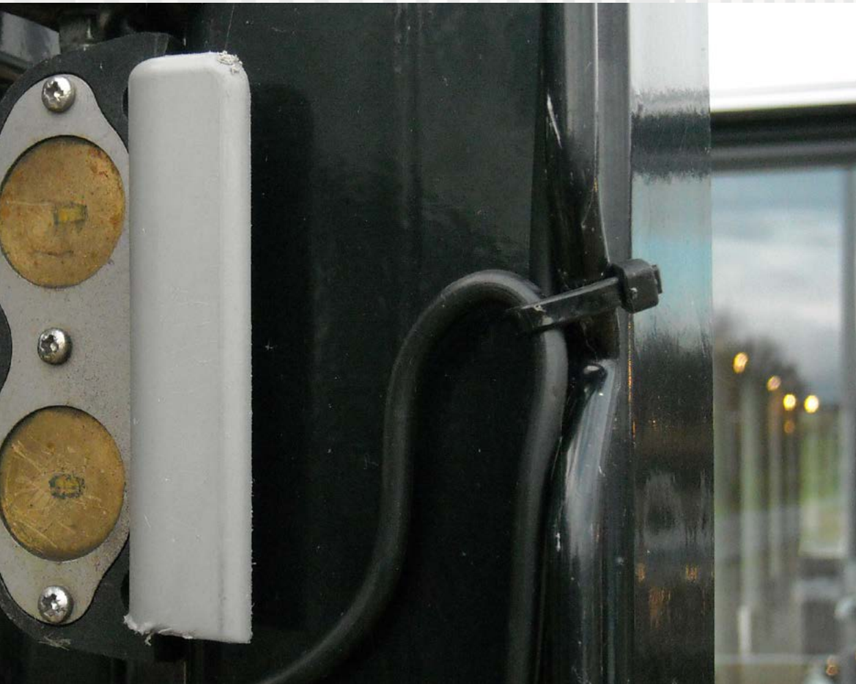
These contacts are used to transfer the voltage to the moving leaf of a swing or sliding gate
