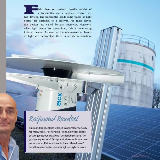
There are also variations on both techniques, consisting of just a single device. With microwave technology, we then refer to a radar. The transmitter and receiver are located in the same housing. With light, we call this a laser detection system. In this situation, too, the transmitter and receiver are located in the same housing: the laser scanner.
